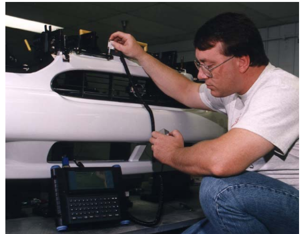
The 3053 can be used with gap and flush gages for assembly line quality audits.
